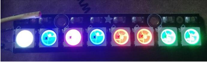
Figure 4 The LEDs stick with their respective colors
