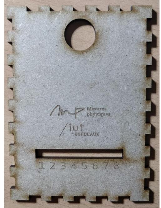
Figure 6 The top plate with the LEDs hole and sensor hole
