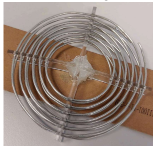
Fig. 4.2.B.5 : Final receiving resonant coil.
