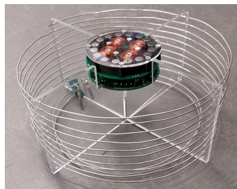
Fig. 4.1.B.3 : Final emitting coil.
