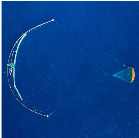
Plastic capture system. (The Ocean Cleanup)
