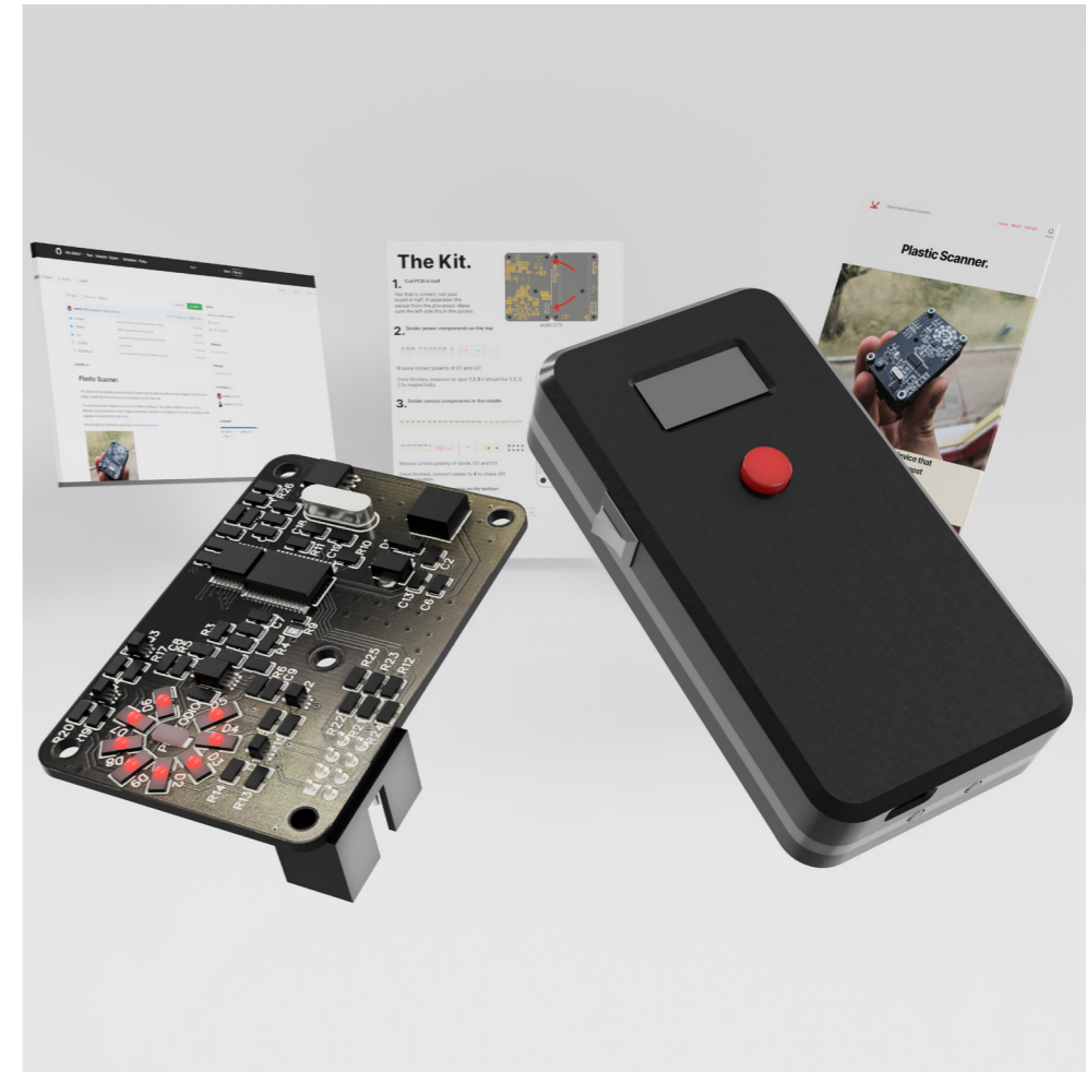
Figure 1: Overview of open-source ecosystem, from left to right: documentation, breakout board, kit, handheld scanner, and website.
