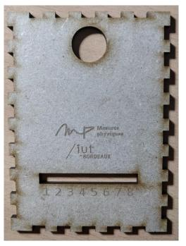
Figure 6 The top plate with the LEDs hole and sensor hole
