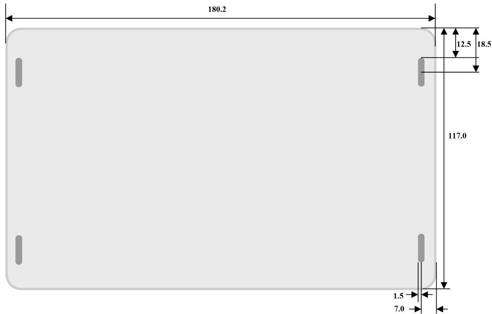
Fig.2-1 Mainboard installation dimension drawing
